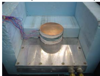
Figure 5: thermal baths to measure thermal conductivity
