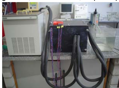
Figure 5: thermal baths to measure thermal conductivity
